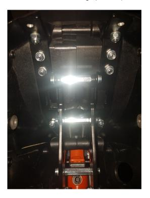
Now you can use the washers and the self-looking nuts to finally fix your cockpit! If you are going to install a STHEADPOD as well leave the nuts and install the STHEADPOD first.
