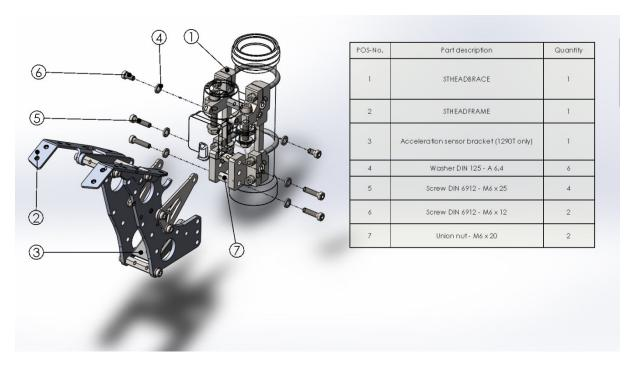
After attaching the STHEADFRAME 2.0 to the STHEADBRACE 2.0 is a good moment to sort out all the wiring before installing both cockpit housing parts.
