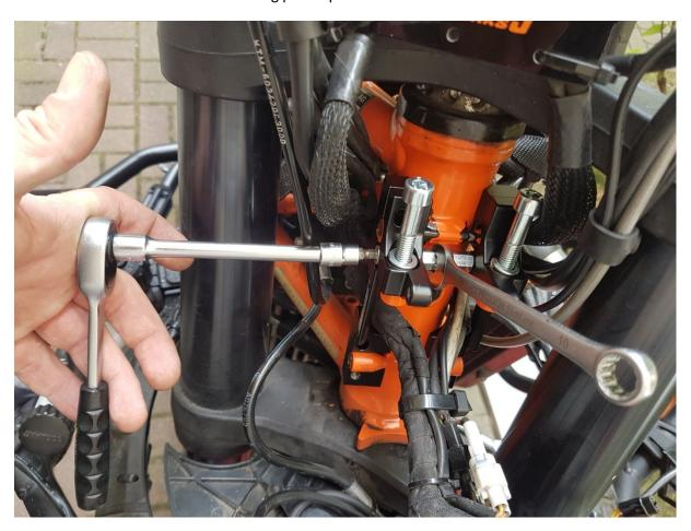
Now fix the bottom block by using the previous M6x25 screws:
