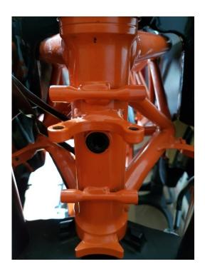
Take the STHEADBRACE and disassemble one half by loosen the bottom block and one side screw:
