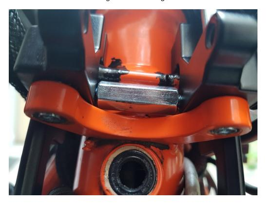
Now insert the steering lock and screw in the M8x50 screws and fix the lock with the M8 self-locking nuts:
