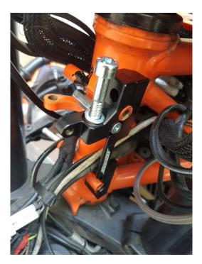
Take now the other half upper part and place and fix it on the other side using the other prepared M8x50 screw and the M6x25 screw. Place the wiring harness between STHEADBRACE 1.0 and the steering head. Leave it outside, if you are using the STHEADBRACE 2.0
